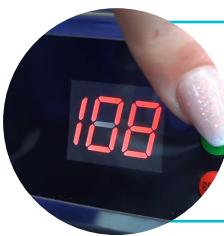
Press the device and set the temperature to 108 degrees. The distiller will now start distilling. Don't forget to check whether the glass jug is positioned correctly under the exhaust filter. Within half an hour the first distilled water will drip from the jug. Within 4 hours the jug will be filled with water and the distiller will give the message 'E', so you know that the basin is empty and the process has been completed.
